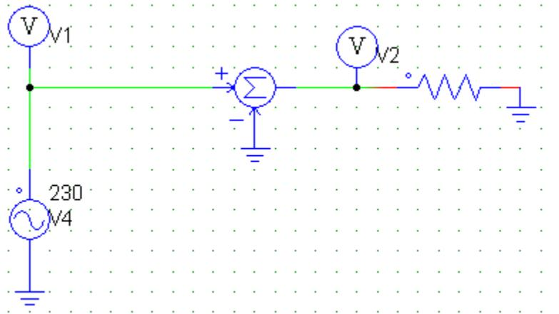
Fig. 1: Electric scheme of direct regulation method with no feedback
