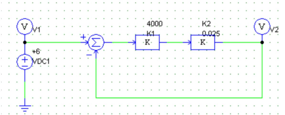
Fig. 3: Scheme of the model of the negative feedback control circuit without influence of external factor
