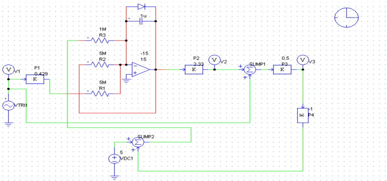
Fig. 6: Operating scheme of the feedback and controlled interference regulation method
