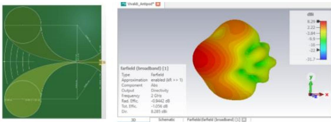
Fig. 5 - PCB antenna and simulation of the far field radiation diagram of a Vivaldi Antenna for a Ground Penetrating Radar.
