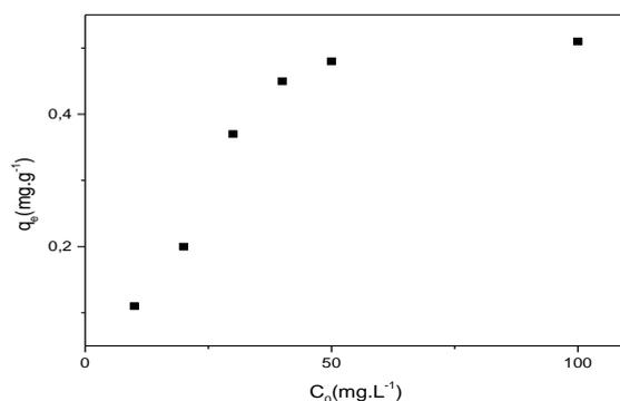
Fig. 4. Effect of the initial concentration of RG12 on the adsorption capacity
