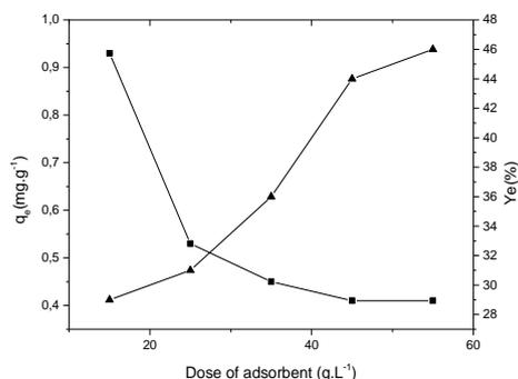
Fig. 3. Effect of adsorbant dose on RG12 adsorption :  $q_e$  ( $\blacktriangle$ ) ,  $Y_e$  ( $\blacksquare$ )
