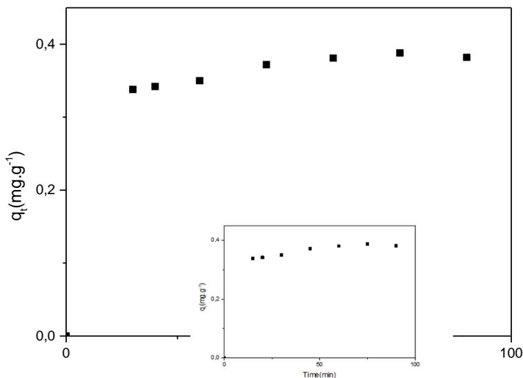
Fig 1. Variation of RG12 adsorbed amount versus time
