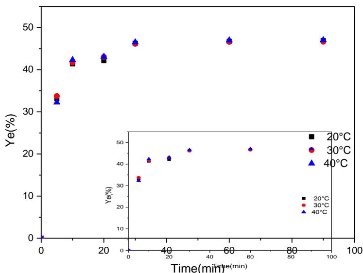
Fig. 5. Effect of temperature variation on yield elimination of RG12 (pH = 5.93, [RG12] = 50mg.L<sup>-1</sup>, m<sub>ads</sub> = 45g.L<sup>-1</sup>).
