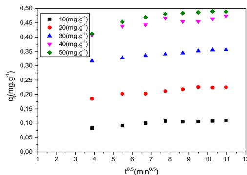
Fig. 7. intra-particle model for adsorption of RG12 on adsorbent
