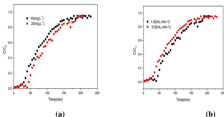
Fig. 8. Breakthrough curves of : (a) RG12 initial concentration, (b) Flow rate and
