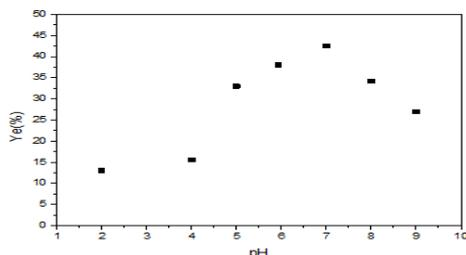
Fig. 3. Effect of the initial pH on the RG12 elimination
