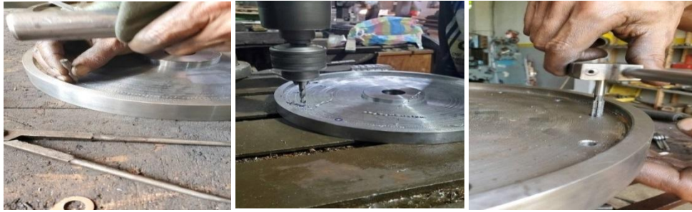
Photo 4: Process of the M8 holes
