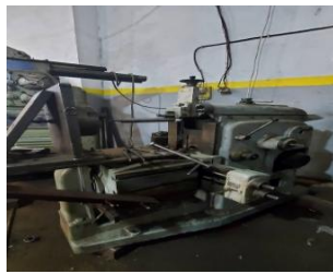
Photo 6: Keyways machine in the workshop
