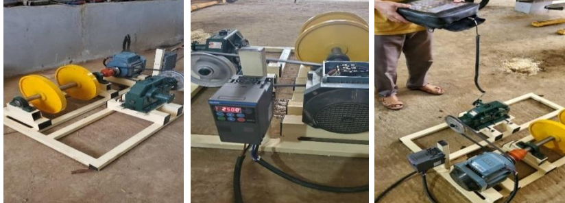
Photos 26, 27, 28 respectively: test bench, Test bench working and test bench under vibration testing under 25Hz
