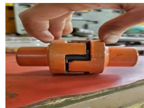
Photo 10: The first state of our coupling (without the mounting holes) photo 5 the final state of our coupling (ready for the mounting)
