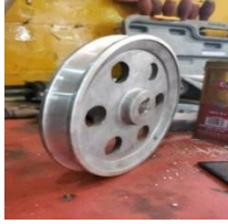
Photo12: Driven pulley 160mm
