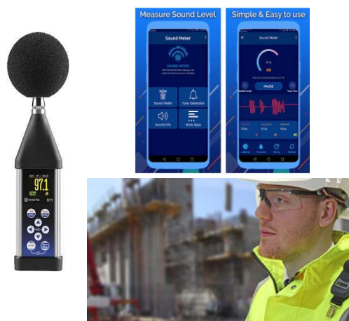
Fig. 1: Examples of devices for measuring the sound. Sound Level Meter (left most), Noise Dosimeter (right down) and Apps for mobile (left up).
